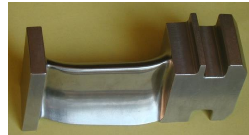
500 MW first stage ODS steel blade
